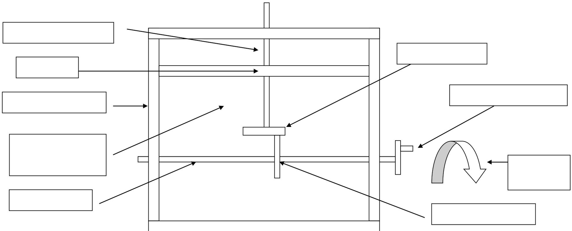
Useful words: cam, movement, linear motion, rotary motion, off-centre, crank handle, axle, frame structure, cam mechanism, cam follower
